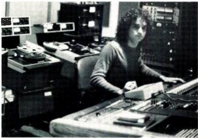
In audio room at National Video Center, audio engineer Roy Yokelson uses Q-Lock to synchronize (left to right) JVC 3/4-inch VTR, two Ampex ATRs, MCI 24-track ATR (out of sight at right).
