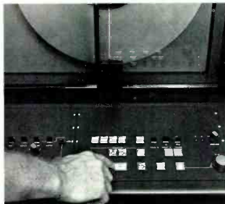
Convenient film deck controls include speed, mode, direction, format, framing, and focus. Adjacent decks control audio, video, and color correction.
